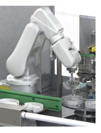
The Robotic Assembly System receives the two components of the assembly from the moulding machines and places them onto shuttles. The parts are then picked using precision-constructed pick heads mounted on two ABB IRB120 robots; they are then accurately assembled within a rotating jig, where they are pressed to lock together, and ejected onto a conveyor.
